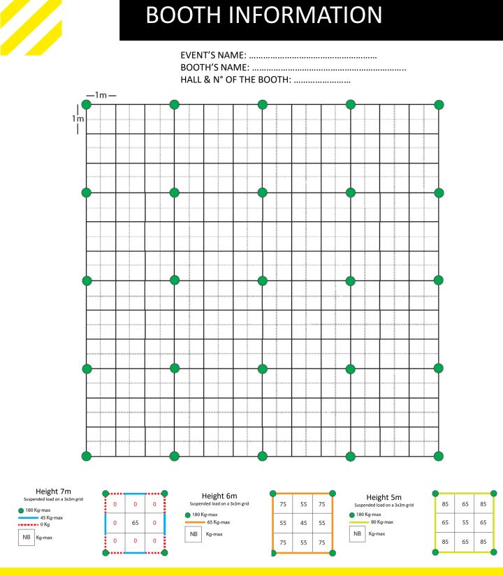
In case of accumulation with 2 hooks on the same anchor point, the weight must be divided by 2.
